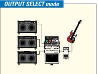
This setup lets you choose between two or three outputs such as switching from a tube amp to a transistor amp to a monster stack, etc.
