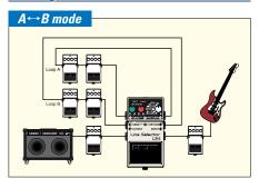
Effects you use for your backing sound are connected to Loop B, while Loop A is used for solos and riffs.
