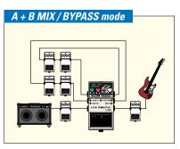
This setting lets you mix a solo sound on Loop A and a backing sound on Loop B.
