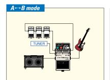
This setup is for switching between an effects loop and tuner. Switch to mode B during live performance for silent tuning.
